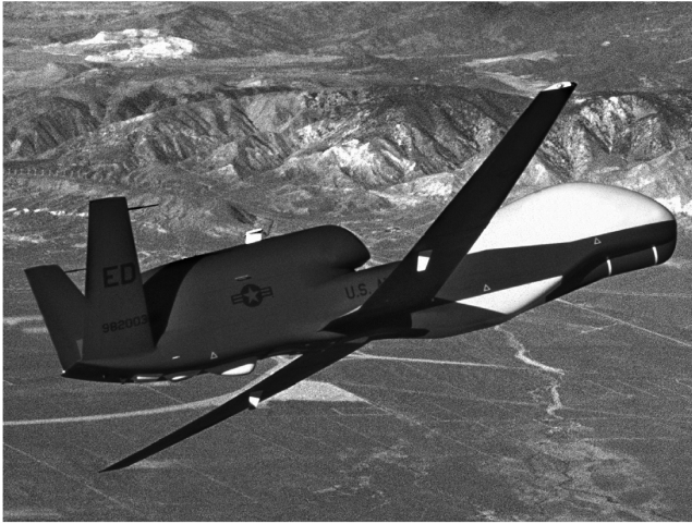
Fig. 2 Example of a V-tail used on the Global Hawk UAV (U.S. Air Force photograph).
